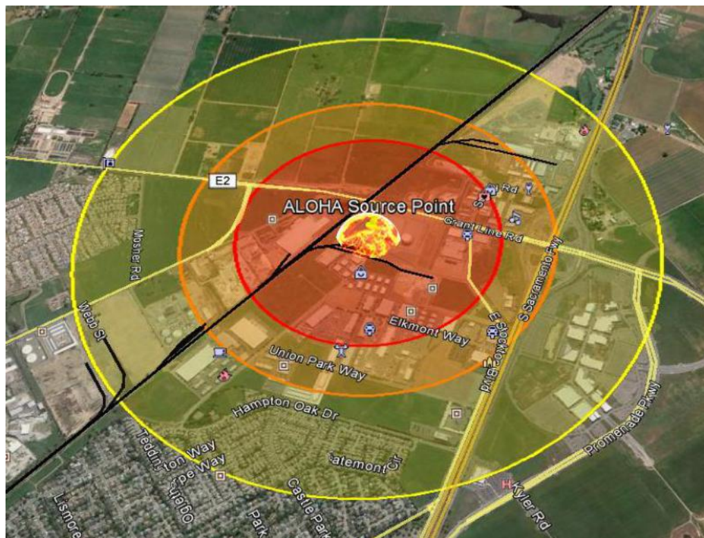
Figure 3: A Google Earth overlay showing one credible scenario had the terrorist plot that targeted the Suburban Propane facility in Elk Grove, California, not been neutralized by the FBI in 1999. It shows thermal threat zones modeled for a boiling liquid expanding vapor explosion in just one of four 60,000 gallon pressurized propane bullet tanks , at the facility. The resulting fireball would have engulfed most of the facility, and the thermal radiation effects would have extended \frac{3}{4} of a mile. If you look to the RH edge of the fireball, below the “e” in “Source,” one of the facility’s two 12-million gallon refrigerated propane storage tanks can be seen on the RH edge of the fireball which would have engulfed most of the site. In a scenario that caused all four bullet tanks to explode nearly simultaneously, the model predicts that the threat zones would extend up to 50% further. Not shown in this figure are the additional effects of overpressure blast wave, and the missile ejection of shrapnel (tank fragments and other debris), which could credibly puncture the large tanks, leading to potentially even larger consequences, which at the very least could cause a large pool fire and deflagration extending well beyond the boundary of the facility. Ironically, the Elk Grove fire station is within the yellow threat zone (the red dot toward the top RH corner of this map). (Fireball diameter 308 yards; Red zone radius: \frac{3}{8} mile [ 10 \text{ kW/m}^2 ] potentially lethal in less than 60 seconds; Orange zone radius: \frac{1}{2} mile [ 5 \text{ kW/m}^2 ] 2 nd -degree burns in less than 60 seconds; Yellow zone radius: \frac{7}{8} mile [ 2 \text{ kW/m}^2 ] pain in less than 60 seconds)
