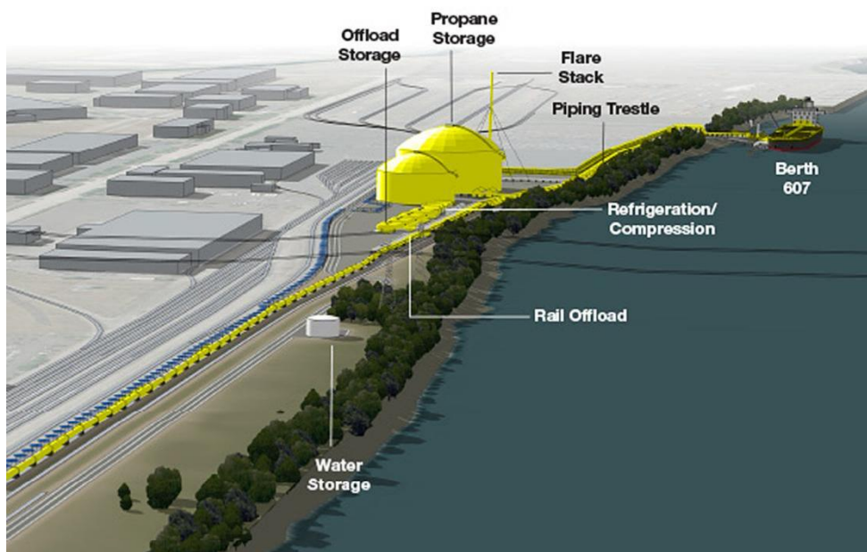
Figure 2: The two double-walled steel refrigerated storage tanks proposed by Pembina for Terminal 6, Portland, OR are of unequal size. The larger tank is 130 feet tall, dwarfing nearby trees. Shown, in front of the storage tanks, are eight 125,000 gallon pressurized bullet transfer tanks. Also shown, stretching diagonally across the picture is a 100 car unit propane train. Propane storage, plumbing, and transportation are shown with yellow highlighting.
